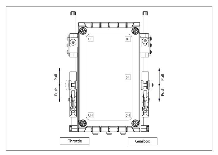
You must program 5 positions and therefore 5 parameters: 2 for the throttle and 3 for the gearbox. Gearbox and throttle positions have to be set according to the parameters of the here below table.
