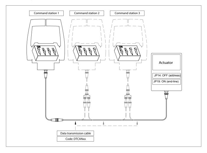
The actuator is placed at one end of the CANBus network.
