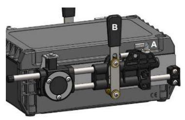
plunger device "A" is positioned as shown in the picture on the left. In emergency situation, to unlock the mechanism it is enough to rotate of 180° the plunger "A" from its working position. After this operation, the mechanism (and the related push-pull cable) can be operated manually using lever (B).
