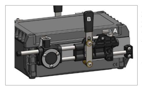
Emergency levers are fitted on the control box. During the normal functioning, the indexing plunger device "A" is positioned as shown in the picture on the left. In emergency situation, to unlock the mechanism it is enough to rotate of 180° the plunger "A" from its working position. After this operation, the mechanism (and the related pushpull cable) can be operated manually using lever (B).
