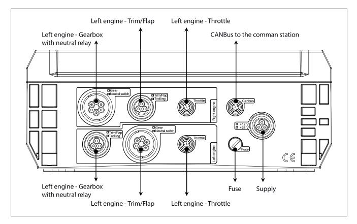
Important: in case of single engine installation, use only the connectors for the right engine.
