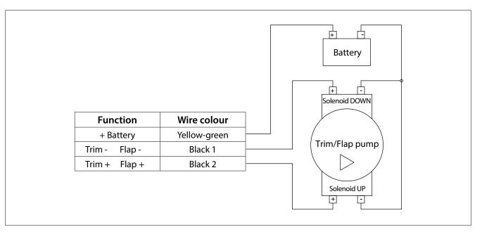
**Important:** this scheme shows how to connect the electrical cables; battery switch and protection devices (e.g. fuses) must be implemented according to local regulations.
