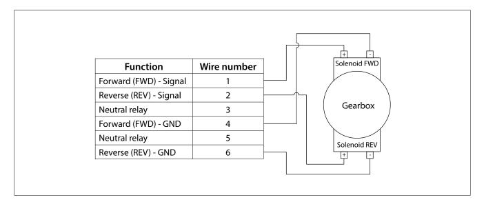
**Important:** this scheme shows how to connect the electrical cables; battery switch and protection devices (e.g. fuses) must be implemented according to local regulations.
