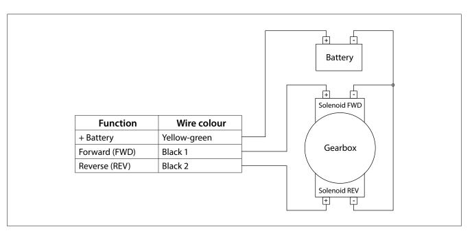
**Important:** this scheme shows how to connect the electrical cables; battery switch and protection devices (e.g. fuses) must be chosen according to local regulations.
