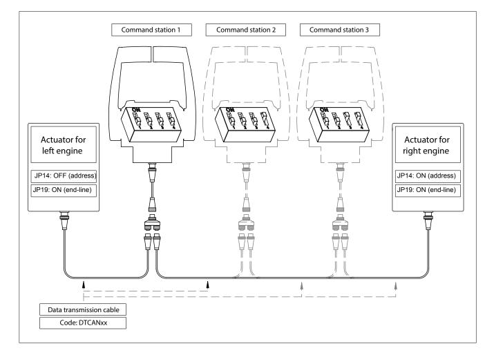
Actuators are placed at the ends of the CANBus network
