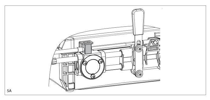
6. Fix the black aluminium cube (e) against the bracket (d) using the fixing screw (c).
