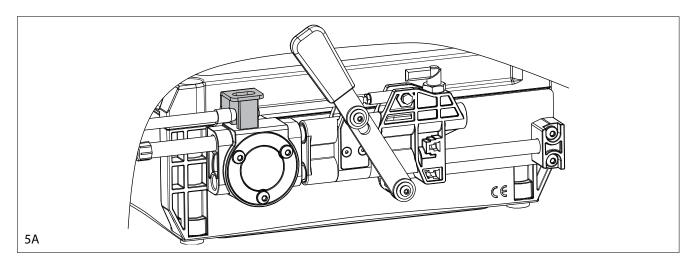
6. Fix the black aluminium cube (e) against the bracket (d) using the fixing screw (c).
