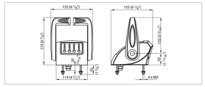
**Important**: in case the screws to fix command station to the dashboard panel are not long enough, don't open the command station to replace them but ask for an adaptation kit.
