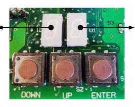
An "E" or "P" will be shown on the side of the actuator with the cable overload error or the cable positioning error
