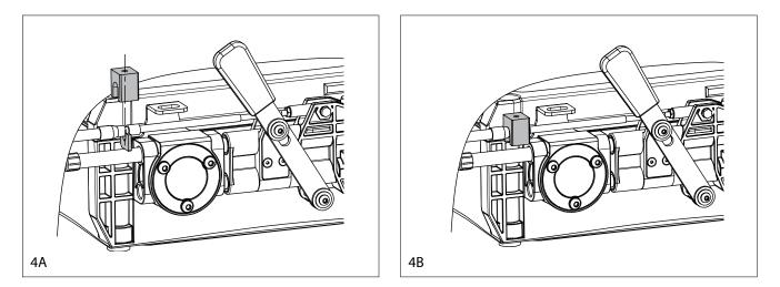
5. Insert the push-pull cable into the slot of the bracket (d). Check that the fixing cube is centred with respect to the slot on the bracket.
