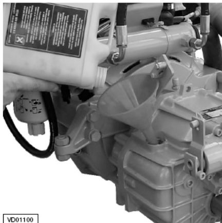
VD01100 Filling with new oil
