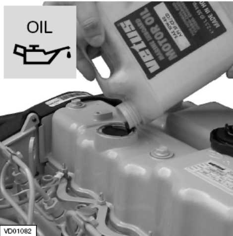
Filling with engine oil
