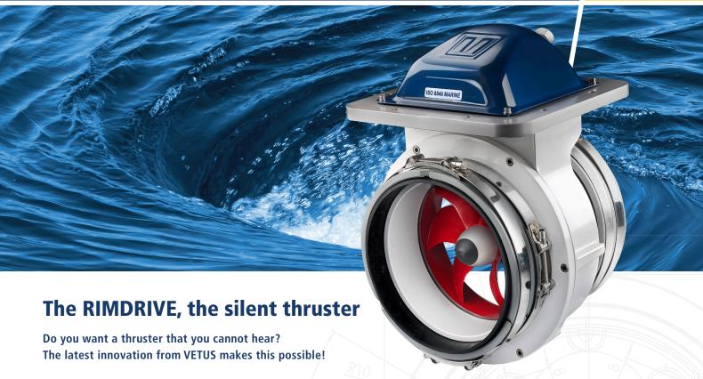
There are two main reasons why the RIMDRIVE is silent. Firstly, the propeller forms the rotating part of the electric permanent magnet motor and therefore noisy gears are not used in this design. Secondly, a ring mounted around the propeller, prevents the propeller tips from cutting through the water. In other words, it prevents cavitation and noise! The proportional speed control also helps to prevent cavitation.
